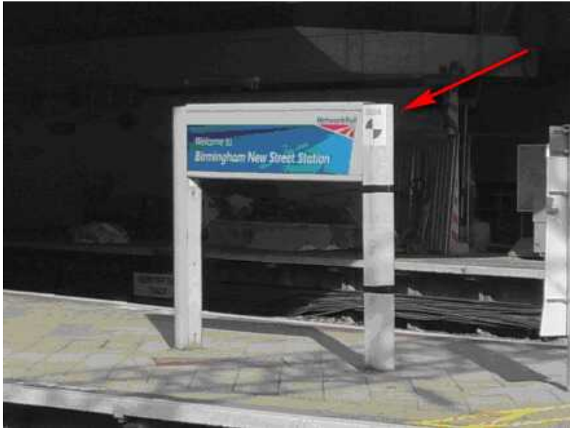
Figure 6: Laser Target 5009 visible on the end of 'Welcome to Birmingham New Street Sign'
