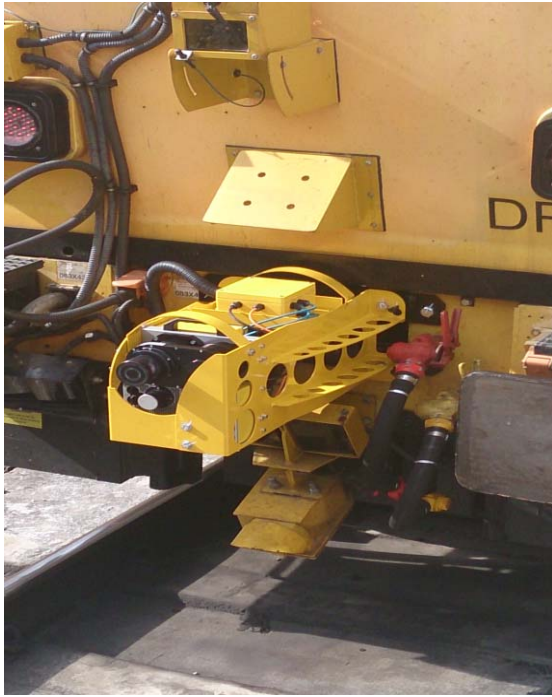
Figure 5: Laser Scanner Install on MPV
