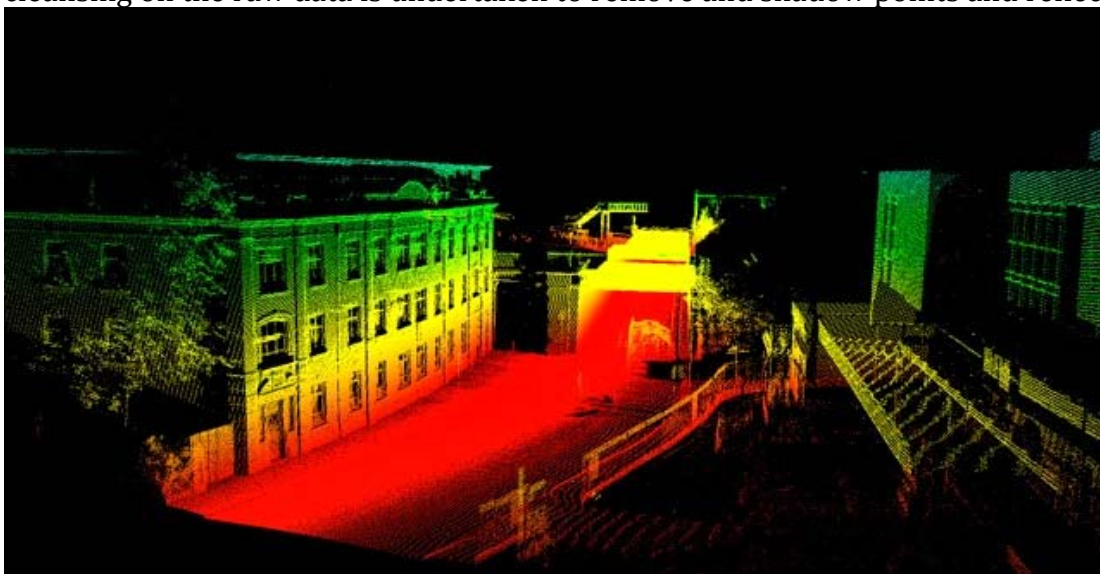
Figure 8: Raw Point Cloud Data
